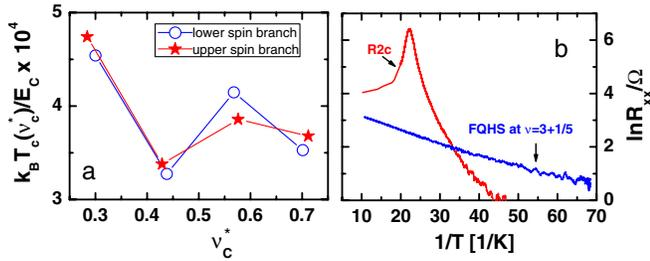
FIG. 4 (color online). The variation with the filling factor  $\nu_c^*$  of the reduced onset temperatures  $T_c(\nu_c^*)/E_C$  at the center of the RIQHSs in the SLL [panel (a)]. Lines are guides to the eye. Arrhenius plot for  $R_{xx}$  and for the  $\nu = 3 + 1/5$  FQHS [panel (b)].
