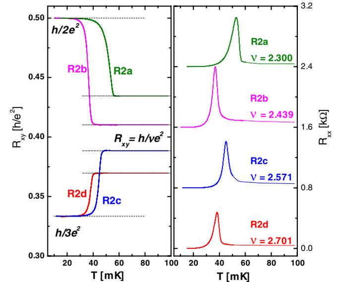
FIG. 2 (color online). The evolution of the magnetoresistance of RIQHSs of the lower spin branch with temperature near the center  $\nu_c$  of each RIQHS. For clarity,  $R_{xx}(T)$  curves are shifted vertically by 0.8 kΩ.
