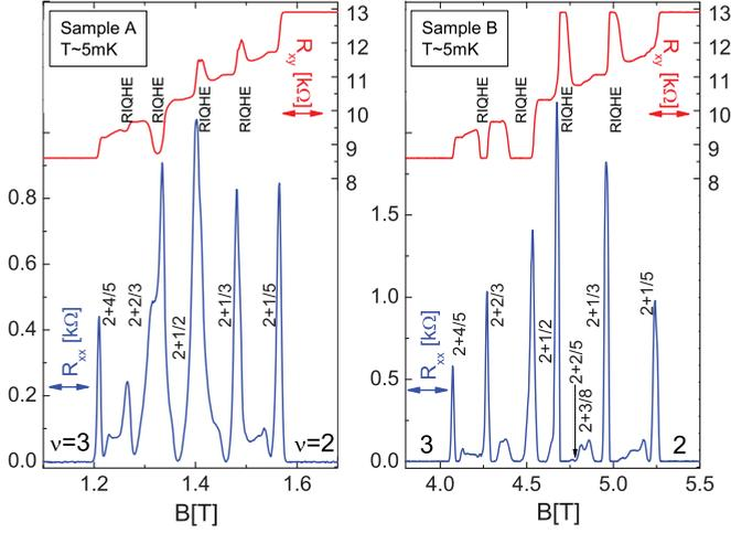
FIG. 1. (Color online) Magnetotransport data in the region of the upper spin branch of the second Landau level. We mark the filling factors  $\nu$  of the observed FQHSs and the reentrant integer quantum Hall states (RIQHSs). Note the vastly different densities of the two samples.
