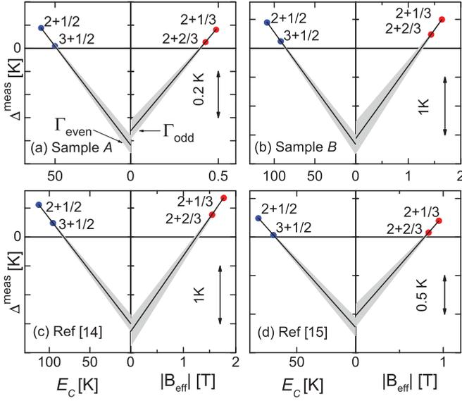
FIG. 3. (Color online) Comparison of the two methods of estimating the disorder parameter  $\Gamma$  for the four analyzed samples. The measured gaps of the even denominator FQHSs extrapolate to  $\Gamma_{\text{even}}$  at  $E_C = 0$ , while those of the  $\nu = 2 + 1/3$  and  $2 + 2/3$  FQHSs to  $\Gamma_{\text{odd}}$  at the vanishing absolute value of  $B_{\text{eff}}$ . The gray shadow is the estimated error for  $\Gamma$ 's.
