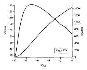
Fig. 2 Transconductance and drain current of device shown in Fig. 1 at drain-source voltage of 15 V
