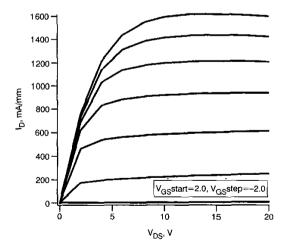
Fig. 1 DC I–V characteristics of  $0.2 \times 25 \ \mu m$  HEMT Source-drain spacing 2  $\mu m$
