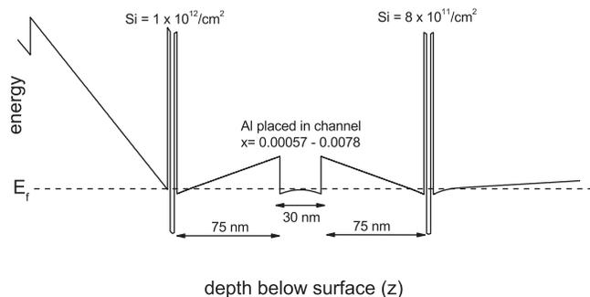
FIG. 1. A schematic band structure of the samples used in this study. Note that the Si dopants are placed in narrow GaAs quantum wells 75 nm above and below the principal 30 nm quantum well.<sup>37</sup>
