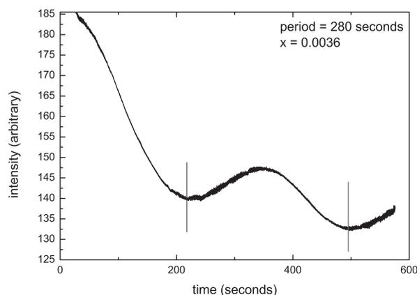
FIG. 2. Plot of RHEED oscillations for Al concentration of  $x = 0.0036$ . The large drop in intensity seen at the start of the data collection is characteristic of AIAs oscillations in our machine. The vertical lines represent deposition of one complete monolayer of AIAs.
